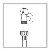
1. Connect the inlet hose by screwing it to a cold water tap using a 3/4 threaded connection (see figure).
