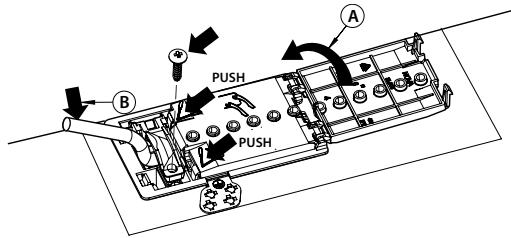
**The appliance must be connected to the electricity supply by means of an all-pole disconnect switch with minimum contact gap of 3 mm.**
