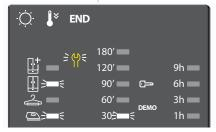
The presence of wrench symbol signals a malfunction. Carry out the operations described. Switch the dryer off and unplug it. Open the door immediately and pull landry out, to allow the heat to dissipate. Wait for about one hour. Reconnect the dryer to the power supply, load the laundry and restart the drying cycle.
