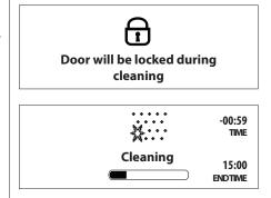
An appropriate message will start flashing on the display once the cycle has finished. The residual temperature will be indicated in the display and the door will remain locked until the temperature inside the oven has returned to a safe level.
