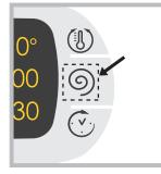
To adjust the settings, gently press the icon inside the sensitive (touch control) area as illustrated in *the figure*.
