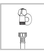
2. Connect the inlet hose by screwing it to a cold water tap using a 3/4 threaded connection (see figure).
