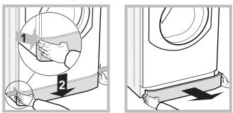
1. take off the cover panel on the front of the machine by first pressing it in the centre and then pushing downwards on both sides until you can remove it (see figures);
