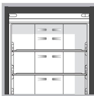
The No Frost system circulates cold air continuously to collect humidity and prevent ice and frost formation. The system maintains an optimal humidity level in the compartment, preserving the original quality of the food, preventing the food from sticking together and making defrosting a thing of the past. Do not block the aeration cells by placing food or containers in direct contact with the refrigerating back panel. Close bottles and wrap food tightly.
