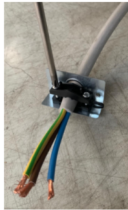
Fix power cord to the plastic holder.
