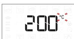
When the °C/°F icon flashes on the display, turn the knob to change the value, then press
