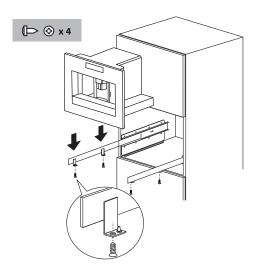
If machine alignment requires adjustment, position the spacers provided either below or at the side of the support.
