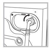
2. Connect the inlet hose to the washing machine by screwing it onto the corresponding water inlet of the appliance, which is situated on the top right-hand side of the rear part of the appliance (see
