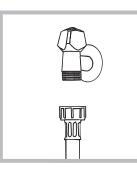
1. Connect the inlet hose by screwing it to a cold water tap using a 3/4 gas threaded connection (see *figure*). Before performing the connection, allow the water to run freely until it is perfectly clear.
