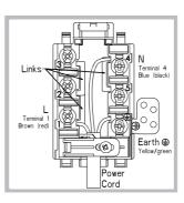
2 Loosen the cable clamp screw and remove it, using a screwdriver as a lever (see figure).
