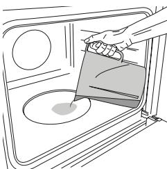
Only when the oven is cold, fill the embossing of the cavity with the quantity of drinking water suggested in the relative cooking table. Place the food in the oven. Set and activate the steam ·
