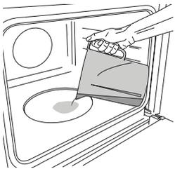
Only when the oven is cold, fill the embossing of the cavity with the quantity of drinking water suggested in the relative cooking table. Place the food in the oven.
