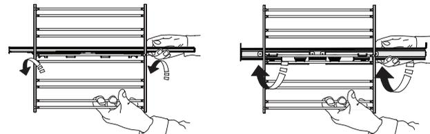
Please note: The sliding runners can be fitted on any level.
