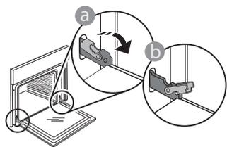
• To remove the door, open it fully and lower the catches until they are in the unlock position.
