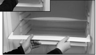
To remove, ensure that the door is open fully. Slide the shelf forward and tilt from position.
