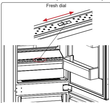
If the crisper is full, the fresh dial located in front of the crisper should be opened. This allows the air in the crisper and the humidity rate to be controlled, to increase the life of food within.
