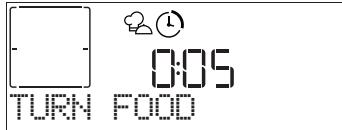
An audible signal will sound and the display shows the action to be done. Open the door, do the action prompted by the display and close the door and resume cooking.
