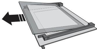
3. Refit the intermediate pane (marked with "R") before refitting the inside pane: To position the panes of glass correctly, make sure that the "R" mark can be seen in the left-hand corner. First insert the long side of the glass marked "R" into the support seats, then lower it into position. Repeat this procedure for both panes of glass.
