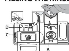
Rinse aid makes dish DRYING easier. The rinse aid dispenser **A** should be filled when the **RINSE AID REFILL** indicator light in the control panel is lit.
