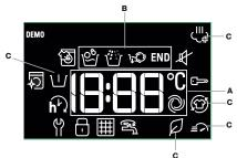
The duration of the available wash cycles and the remaining time of a running cycle appear in section A (the display will show the maximum
