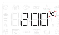
When the °C icon flashes on the display, turn the knob to change the value, then press to confirm and continue to alter the settings that follow (if possible). You can also set the grill level (3 = high, 2 = medium, 1 = low) at the same time.
