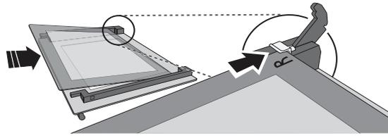
Refit the upper edge: a click will indicate correct positioning. Make sure the seal is secure before refitting the door.
