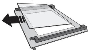
3. Refit the intermediate pane (marked with "1R") before refitting the inside pane: To position the panes of glass correctly, make sure that the "R" mark can be seen in the left-hand corner. First insert the long side of the glass marked "R" into the support seats, then lower it into position. Repeat this procedure for both panes of glass.
