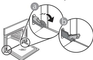
2. Close the door as much as you can. Take a firm hold of the door with both hands – do not hold it by the handle. Simply remove the door by continuing to close it while pulling it upwards at the same time until it is released from its seating. Put the door to one side, resting it on a soft surface.
