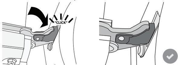
5. Try closing the door and check to make sure that it lines up with the control panel. If it does not, repeat the steps above: The door could become damaged if it does not work properly.
