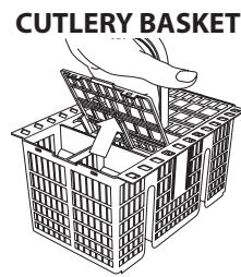
The basket is equipped with top grilles for improved cutlery arrangement. The cutlery basket should be positioned only at the front of the lower rack.
