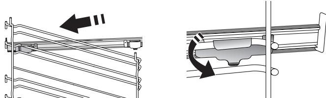
Please note: The sliding runners can be fitted on any level.
