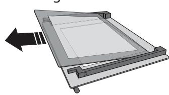
3. Refit the intermediate pane (marked with "R") before refitting the inside pane: To position the panes of glass correctly, make sure that the "R" mark can be seen in the left-hand corner. First insert the long side of the glass marked "R" into the support seats, then lower it into position. Repeat this procedure for both panes of glass.
