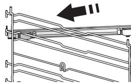
Remove the shelf guides from the oven and remove the protective plastic from the sliding runners.
