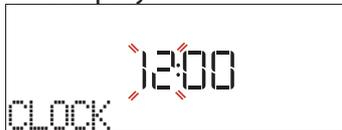
Press + or - to set the correct hour and press ✓: The two digits for the minutes will flash on the display. Press + or - to set the minutes and press ✓ to confirm.
