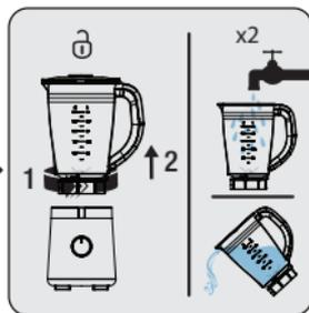
Remove the jug (3) from the motor unit (6). Rinse with water to clean up large food residues that can pile up in the container.
