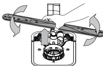
The lower spray arm may be removed by pulling it upwards and rotating it anti-clockwise. Mounting back the spray arm is by pulling it down and rotating it clockwise.
