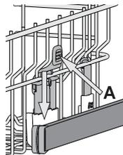
**We strongly recommend that you do not adjust the height of the rack when it is loaded. NEVER raise or lower the basket on one side only.**
