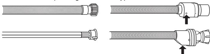
If the inlet hose has a transparent coating, periodically check if the colour intensifies locally. If yes, the hose may have a leak and should be replaced. For water stop hoses: check the small safety valve inspection window (see arrow). If it is red, the water stop function was triggered, and the hose must be replaced by a new one. For unscrewing this hose, press the release button while unscrewing the hose.
