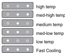
At first plug-in of appliance temperature setpoint is present at medium position (factory setting).
