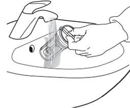
6. Insert the water filter and reinstall the plinth: Reinsert the water filter again by turning it in clockwise direction. Make sure to turn it in as far as it goes; the filter handle must be in vertical position. To test water tightness of the water filter, you can pour about 1 liter of water into the detergent dispenser. Then reinstall the plinth.
