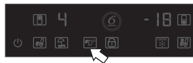
Active 0 compartment off: button partially lighted
