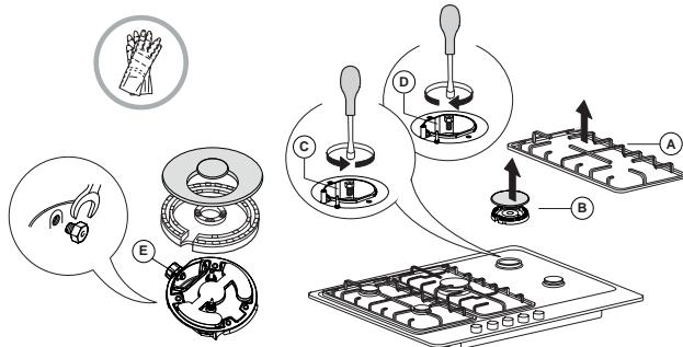
Before installing the hob, remember to affix the gas calibration plate supplied with the injectors in such a way that it covers the existing information relating to gas calibration.
