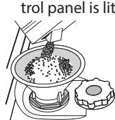
1. Remove the lower rack and unscrew the reservoir cap (anticlockwise).
