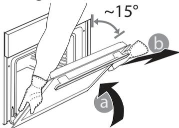
Refit the door by moving it towards the oven, aligning the hooks of the hinges with their seating and securing the upper part onto its seating.
