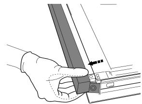
2. Lift and firmly hold the inner glass with both hands, remove it and place it on a soft surface before cleaning it.
