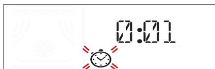
Press **OK select** to activate the timer: An audible signal will sound and the display will indicate once the timer has finished counting down the selected time.
