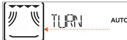
Once the oven has paused cooking, open the door and carry out the action you are prompted to perform before closing the door again and pressing **▶** to continue with cooking.
