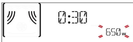
When a setting is flashing on the display, use **▲** or **▼** change it, then press **OK select** to confirm and continue to alter the settings that follow (if possible).
