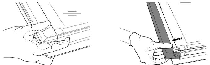
**3. To correctly reposition the inner glass**, make sure that the "R" is visible in the left-hand corner and the clear surface (not printed) is facing up. First insert the long side of the glass indicated by "R" into the support seats, then lower it into position.
