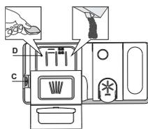
**To open the detergent dispenser use the opening device C. Introduce the detergent into the dry dispenser D only. Place the amount of detergent for pre-washing directly inside the tub.**
