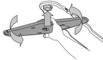
The top spray arm may be removed by pressing it up and then rotating it anti-clockwise. Mounting back the spray arm is by pulling it upwards and rotating it clockwise.
