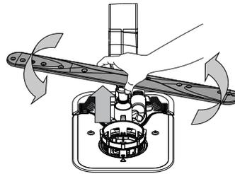
The lower spray arm may be removed by pulling it upwards and rotating it anti-clockwise. Mounting back the spray arm is by pulling it down and rotating it clockwise.
