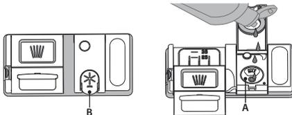
1. Open the dispenser B by pressing and pulling up the tab on the lid.
