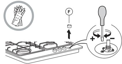
Upon completion of adjustment, reseal using sealing wax or an equivalent material.
