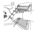
To make best use of the catalytic panels' self-cleaning properties, we recommend heating the oven to 200 °C for around one hour using the "Convection Bake" function. The oven must be empty during this time. Then leave the appliance to cool down before removing any remaining food residues using a nonabrasive sponge.
