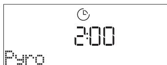
Press + or — to select the desired cycle, then press  to confirm. Once a cycle has been selected, if desired, press + or — to set end time (start delay), then press  to confirm.
