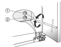
5. Use the wrench provided (if present) to adjust the levelling bolts. Turn clockwise to raise the appliance, or anticlockwise to lower it. It may take several turns of the levelling bolts and/or feet to adjust the tilt of the refrigerator.
