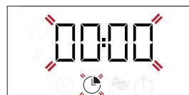
Use or to set the cooking time you require, then press to confirm. Activate the function by turning the *thermostat knob* to the temperature you require: an audible signal will sound and the display will indicate that cooking is complete.
