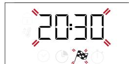
Use or to set the time you want cooking to end and press to confirm. Activate the function by turning the *thermostat knob* to the temperature you require: the function will remain paused until it starts automatically after the period of time that has been calculated in order for cooking to finish at the time you have set.
