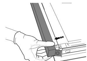
**3. To correctly reposition the inner glass**, make sure that the "R" is visible in the left-hand corner and the clear surface (not printed) is facing up. First insert the long side of the glass indicated by "R" into the support seats, then lower it into position.
