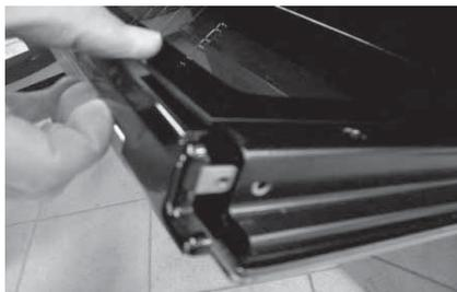
Gently ease the glass upwards and remove from the door. Repeat with the centre door glass (if fitted)
