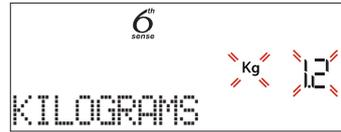
To set the function correctly, follow the indications on the display, when prompted, and press + or - to set the required value then press
