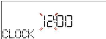
Press + or – to set the current hour and press ✓: The two digits for the minutes will flash on the display. Press + or – to set the minutes and press ✓ to confirm.
