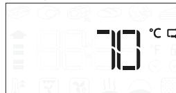
If the meat probe is plugged during the selection of a function, display switches to the default meat probe target temperature.
