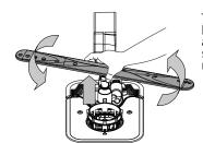
The lower spray arm may be removed by pulling it upwards and rotating it anti-clockwise. Mounting back the spray arm is by pulling it down and rotating it clockwise.
