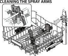
On occasions, food residue may become encrusted onto the spray arms and block the holes used to spray the water. It is therefore recommended that you check the arms from timé to time and clean them with a small non-metallic brush.
