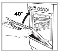
4. Press the two buttons on the upper profile and extract the profile (see photo)
